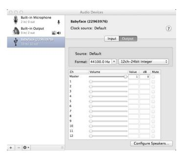
Mac OSX supports USB Audio 2.0, even with more than 2 channels. The Babyface offers full 10 input and 12 output channels at up to 192 kHz. It is shown as "Babyface (xxxxxxxx)" in the Audio MIDI Setup, in both normal and CC mode. In CC mode the USB Settings will vanish from the Dock, and TotalMix will – if at all – show a 'disconnected' Babyface.
