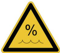
To reduce the risk of fire or electric shock do not expose this device to rain or moisture. Prevent moisture and water from entering the device. Never leave a pot with liquid on top of the device. Do not use this product near water, i. e. swimming pool, bathtub or wet basement. Danger of condensation inside – don't turn on before the device has reached room temperature.
