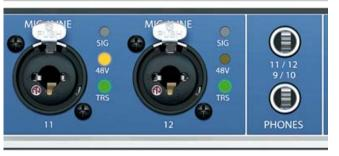
**Phones 2**. These low impedance outputs of highest quality are able to drive headphones at higher levels undistorted, no matter if low or high impedance headphones are used.
