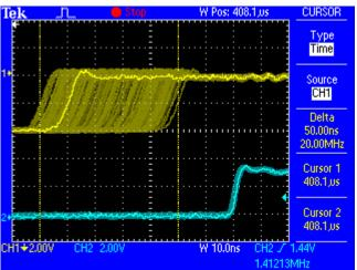
The screenshot shows an extremely jittery SPDIF signal of about 50 ns jitter (top graph, yellow). SteadyClock turns this signal into a clock with less than 2 ns jitter (lower graph, blue). The signal processed by SteadyClock is of course not only used internally, but also used to clock the digital outputs. Therefore the refreshed and jitter-cleaned signal can be used as reference clock without hesitation.
