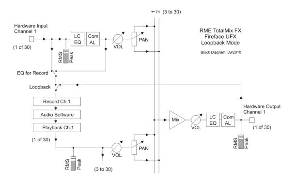
The block diagram shows how the software's input signal is played back, and fed back from the Hardware Output to the software input.
