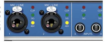
Inputs 3/4, **INST/LINE**, accept both a balanced line signal as well as an unbalanced instrument signal via 1/4" TRS plug.
