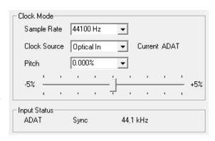
This way, configuring any suitable audio application for digital recording is simple. After selecting the correct input, Fireface UCX displays the current sample frequency. This parameter can then be changed in the application's audio attributes (or similar) dialog.
