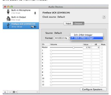
Mac OSX supports USB Audio 2.0, even with more than 2 channels. The UFX offers 22 input and 22 output channels at up to 96 kHz. It is shown as "Fireface UCX (xxxxxxxxx)" in the Audio MIDI Setup, in both normal and CC mode. In CC mode the USB Settings will vanish from the Dock, and TotalMix will – if at all – show a 'disconnected' UCX.
