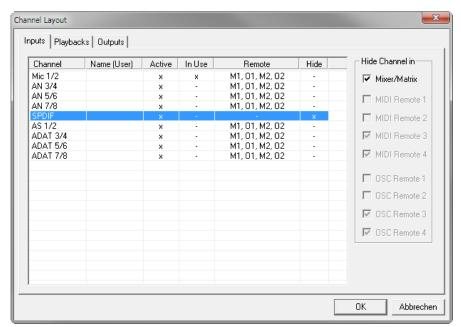
Rows Inputs, Playbacks and Outputs are set up individually by the tabs at the top. *Active* indicates currently available channels. At higher sample rates many ADAT channels are no longer active. *In Use* shows which channels are currently used in the mixing process.
