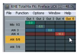
The Matrix not always replaces the mixer view, but it significantly enhances the routing capabilities and - more important - is a brilliant way to get a fast overview of all active routings. It shows you in a glance what's going on. And since the Matrix operates monaural, it is very easy to set up specific routings with specific gains.
