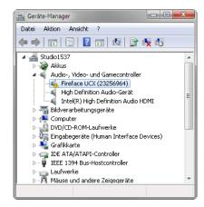
Windows does not support USB Audio 2.0 directly. The UCX will be detected, but automatic driver installation will fail. This is important to remember. Connecting it to the PC one day after having it used with the iPad one might forget that it is still in CC mode. You might end up with hours of wasted time trying to repair your driver installation – when all you need to do is set the unit back to normal mode.
