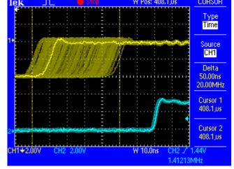
The screenshot shows an extremely jittery SPDIF signal of about 50 ns jitter (top graph, yellow). SteadyClock turns this signal into a clock with less than 2 ns jitter (lower graph, blue). The signal processed by SteadyClock is of course not only used internally, but also used to clock the digital outputs. Therefore the refreshed and jitter-cleaned signal can be used as reference clock without hesitation.
