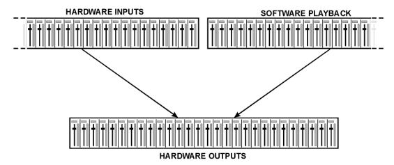
56 channels don't fit on the screen side by side, neither does such an arrangement provide a useful overview. Therefore, the channels have been arranged as known from an *Inline* desk, so that the row *Software Playback* equals the *Tape Return* of a real mixing desk:
