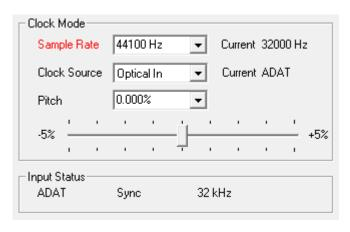
In practice, SyncCheck provides the user with an easy way of checking whether all digital devices connected to the system are properly configured. With SyncCheck, finally anyone can master this common source of error, previously one of the most complex issues in the digital studio world.
