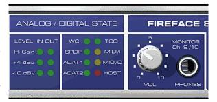
The red **HOST** LED lights up when the Fireface 800 has been switched on, signalling the presence of operating voltage. At the same time it operates as error LED, in case the FireWire connection hasn't been initialised yet, or has been interrupted (error, cable not connected etc.).
