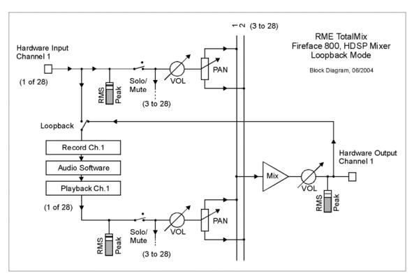
As each of the 28 hardware outputs can be routed to the record software, and none of these hardware inputs get lost, TotalMix offers an overall flexibility and performance not rivalled by any other solution.
