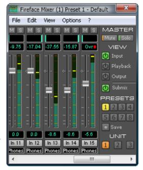
This level display of TotalMix also provides means for a constant monitoring of the signal quality. Thus it can be a valuable tool for sound optimization and error removal in the studio.
