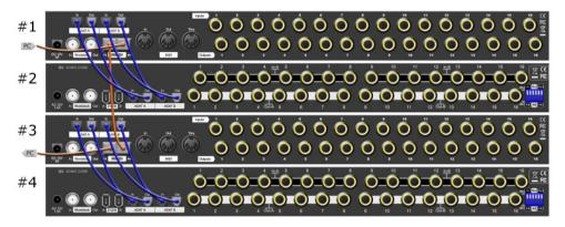
If you own two ADAT converters (in this example the A16 ultra by Sonic Core), you can incorporate them as shown. In doing so, set the routing for the two A16 MK-II as follows:
