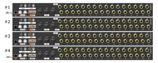
In this example four A16 MK-II are simply chained in row in order to have 2 x 64 channels. For this purpose, set the four A16 MK-II from MADI 1 to MADI 4 in the *routing preset*.
